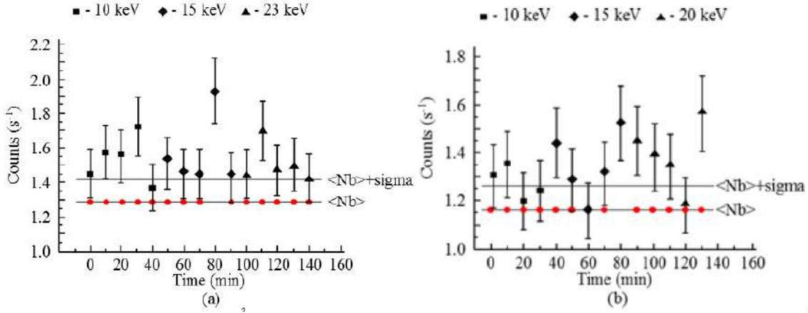
**Figure 9.** Counting rate of the <sup>3</sup>He-neutron detector (■, ◆, ▲). (a) Ti/TiO<sub>2</sub>:D<sub>x</sub> target 300 μm thick and H<sup>+</sup> beam (10, 15, and 23 keV), (b) Ti/TiO<sub>2</sub>:D<sub>x</sub> target 30 μm thick and Ne<sup>+</sup> beam (10, 15, and 20 keV). The average background (Nb) (red filled circles) was measured using the Cu target.
