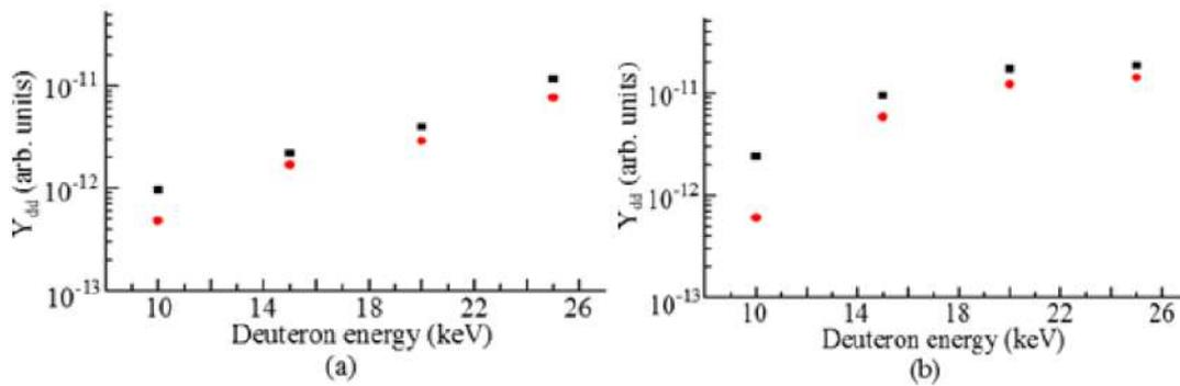
**Figure 6.** Dependence of the DD-reaction yield from the Ti/TiO<sub>2</sub>:D<sub>x</sub> target (left) and from the Pd/PdO:D<sub>x</sub> target (right) on the D<sup>+</sup> beam energy: the measured DD-reaction yield along the beam (■) and the DD-reaction yield calculated for a given energy (red filled circles).
