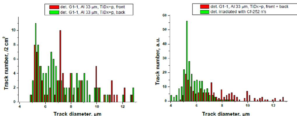
**Figure 8.** *Left* - the diameter distribution of the tracks on the front (red bars) and rear (green bars) side of the detector coated 33  $\mu\text{m}$  Al, located below the sample  $\text{Ti} / \text{TiO}_2:\text{D}_x$ , irradiated by a proton beam with an energy of 23 keV. *Right* - Total tracks diameter distribution of the front and rear sides of the detector (red columns) compared with a detector irradiated by neutrons from the source Cf-252 (green bars).
