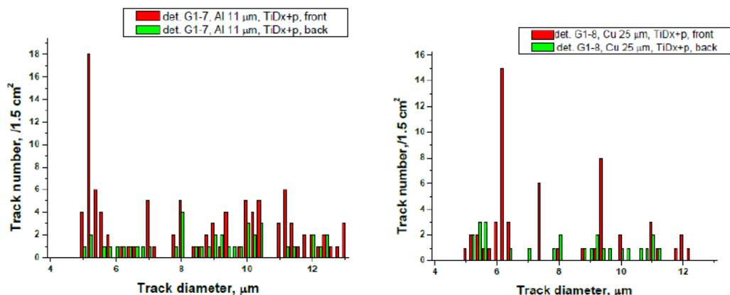
**Figure 7.** Diameter distribution of tracks on the detectors coated 11  $\mu\text{m}$  Al (left) and 25  $\mu\text{m}$  Cu (right), located above the sample  $\text{Ti}/\text{TiO}_2:\text{D}_x$ , irradiated by a  $\text{H}^+$  beam with an energy of 23 keV. Comparison of readings front and back sides of the detectors indicates the presence of proton emission from the DD-reaction.
