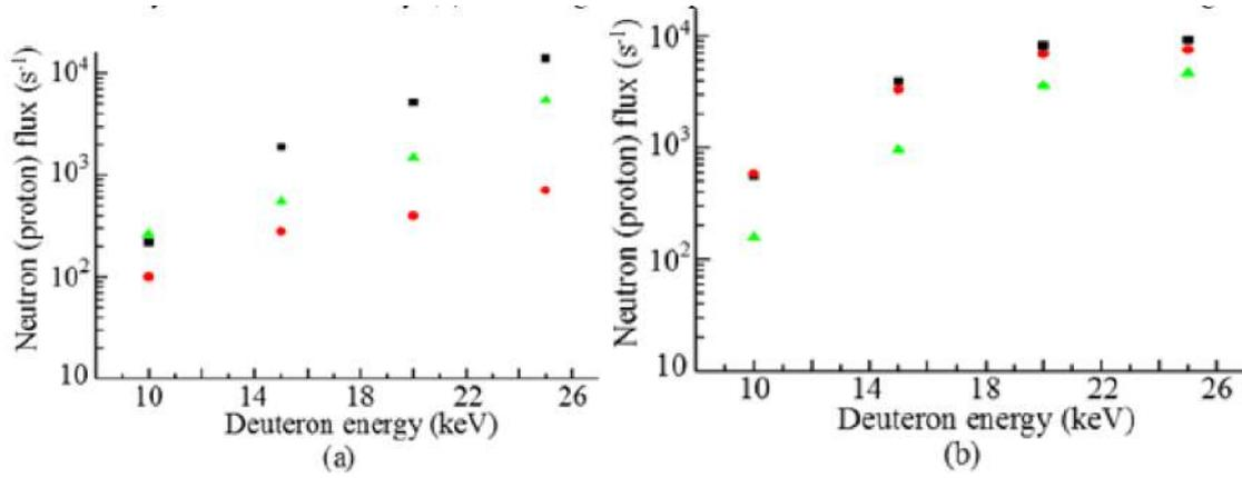
**Figure 5.** The energy dependence of the fluxes of protons and neutrons emitted along and opposite to the beam for Ti/TiO<sub>2</sub>:D<sub>x</sub>(left) and Pd/PdO:D<sub>x</sub> (right) targets. Neutron flux along the beam (■), neutron flux opposite to the beam (red filled circles), and proton flux opposite to the beam (green filled triangles). Measurements were performed by the CR-39 track detector.
