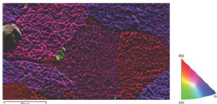
**Figure 4.** FSD and Euler Color Map overlay of palladium foil seen in Fig. 3 using the same Hitachi S4300 instrument.
