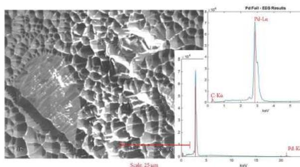
**Figure 3.** SEM and EDS results of a pure palladium electrode using Hitachi S4300 at TTU Imaging Center.
