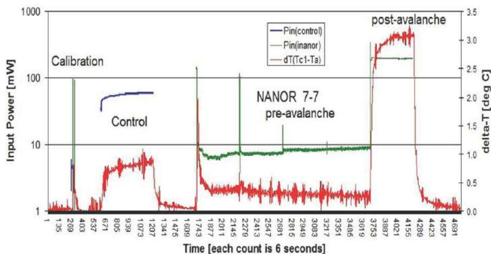
**Figure 3.** Temperature difference induced by a ZrO<sub>2</sub>–NiD NANOR<sup>®</sup>-type component and ohmic control, both electrically driven, showing both excess heat and avalanche behavior.
