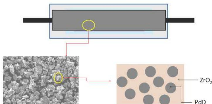
**Figure 1.** A schematic and actual view of an early NANOR<sup>®</sup>-type component. (Top) Shown is the two terminal component with the cylindrical shaped core. (Bottom left) A scanning micrograph shows the nanomaterial in the core. (Bottom right) A schematic illustration of the electrically insulating zirconia within which lie islands of deuterated alloy.
