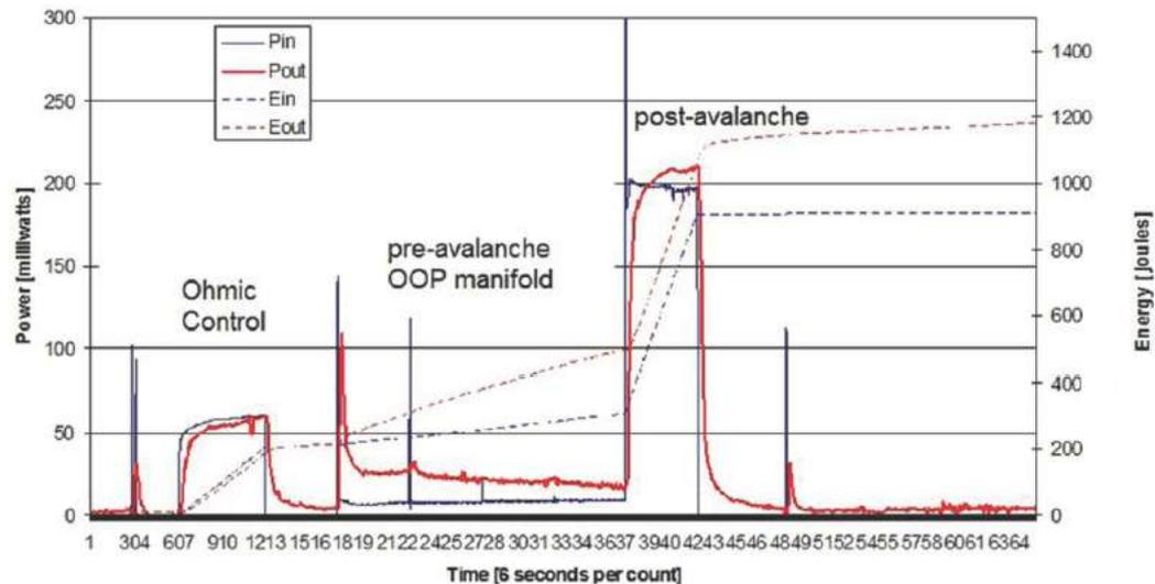
**Figure 5.** Four curves showing the input power and thermal power output, and their time integrals showing both excess heat and avalanche behavior, in a  $\text{ZrO}_2\text{-NiD}$  NANOR<sup>®</sup>-type component.
