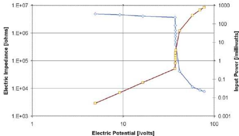
**Figure 2.** Impedance and Electrical current as a function of applied electric potential (volts). This figure shows the response, and particularly the Avalanche behavior with three regions, as first observed with ZrO<sub>2</sub>-NiH NANOR<sup>®</sup>-type component. Three regions are seen; consisting of the initial plateau of electrical impedance, then the rapid fall off, and finally a sloped region at higher voltage [4,1].
