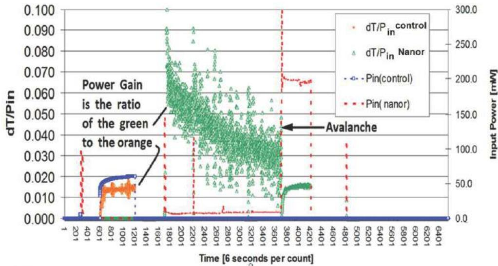
**Figure 4.** These curves show the  $dT/P_{in}$  ratios, which enable determination of the power gain, both in the excess heat region and after the avalanche behavior, for a  $ZrO_2$ -NiD NANOR<sup>®</sup>-type component. The region of the Avalanche is labeled.
