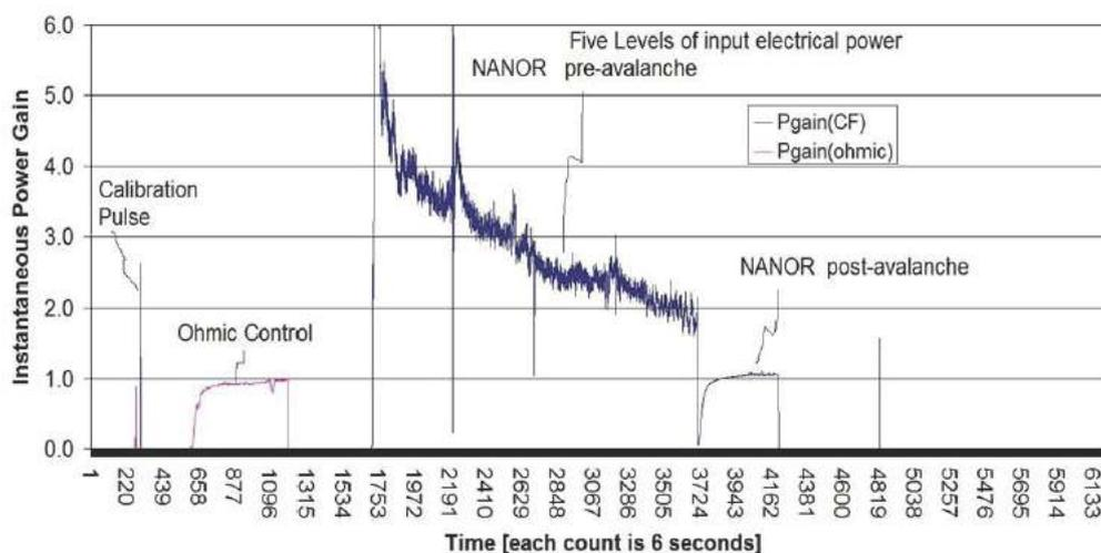
**Figure 6.** This graph presents the power gain of the  $\text{ZrO}_2\text{-NiD}$  NANOR<sup>®</sup>-type component CF/LANR component as a function of time, and shows that the excess heat which is generated decreases with high input power, eventually reverting to normal, ordinary, resistor-like operation after the electrical avalanche.
