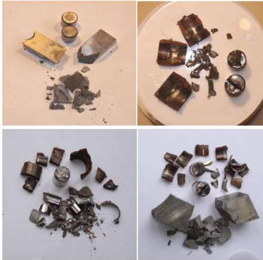
Figure 12. Debris from four strong explosions using calcium deuteride and calcium hydride, which shattered the anvil bearings in three cases and the upper HSS spacer in two cases.
