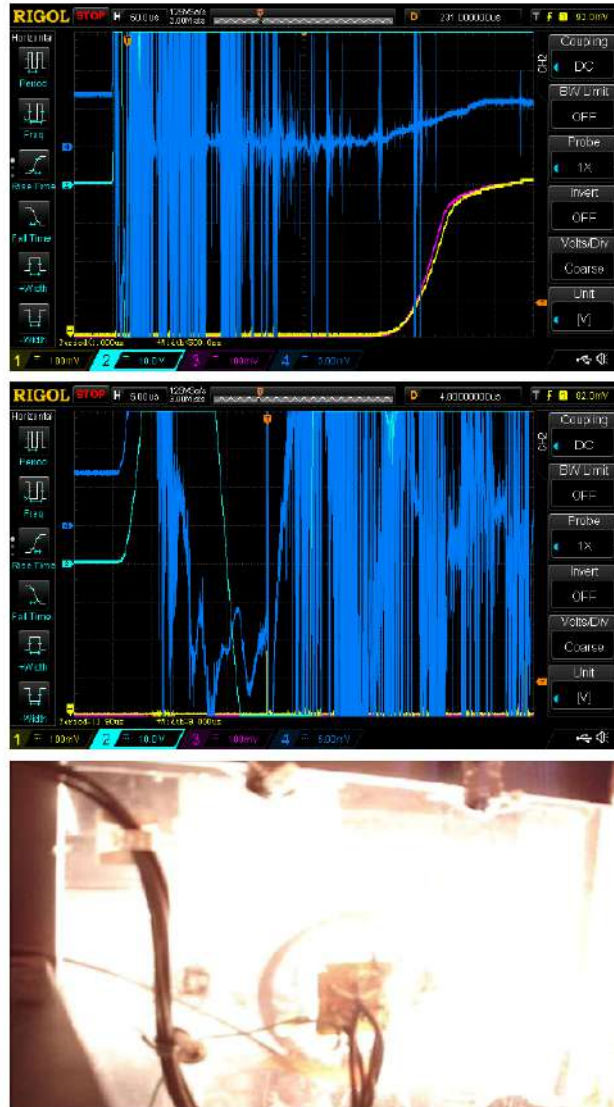
Figure 4. Oscilloscope traces for one very strong explosion, shown at 50 and 5 \mu s/division temporal resolution (use zoom 200% to view details). Blue trace is the load-cell output showing how the press applied load at 20 tons is increased above 40 tons by the explosion lasting only for 8 \mu s, followed by total fall-off and strong mechanical ringing. Turquoise trace is the output from the piezo-accelerometer, which was attached to the side of the cell until it burst. Yellow trace illustrates the response of the direct view photodiode to the debris ignition, and red trace the output from the photodiodes with UV scintillators. There is some cross-talk between the four channels because of amplifier overload. The over-exposed video camera recording of the bright explosion flash was viewed through a 12 mm thick shatterproof polycarbonate window; see Fig. 9 for mechanical layout details. The photodiodes, shown with wires attached mounted in the centre of the polycarbonate window, view through a hole but are protected from flying debris by a stainless steel mesh. Picture width corresponds to 200 mm \times 120 mm high.
