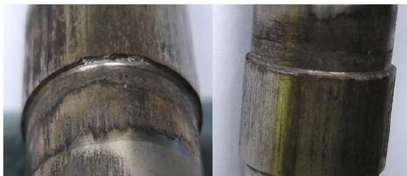
Figure 14. Enlarged view of two typical results of fusion ignition wherein the explosion gas pressure has broken pieces off the piston shoulders, in order to escape upwards.
