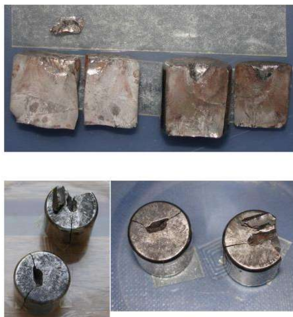
Figure 3. Two typical results of fusion ignition, wherein the local gas pressure has forced a wedge of steel downwards through the lower bearing, splitting it apart. One of the wedges is shown at top left, and sitting on the appropriate bearing in the lower views. It is triangular in cross-section, roughly 4 mm \times 1 mm \times 2 mm deep.
