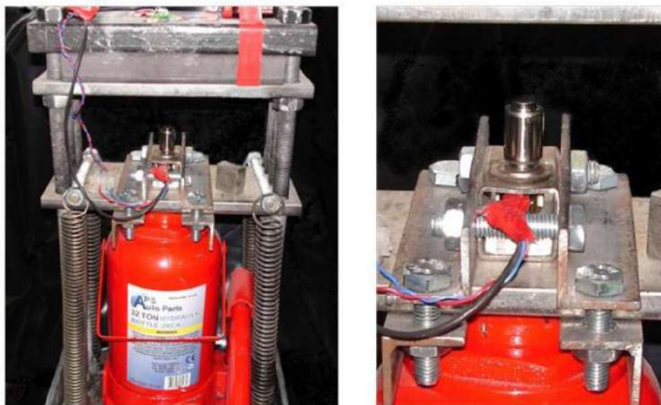
Figure 8. Left: photograph of bottle-jack press assembly. Right: close-up view of fusion cell standing on load-cell assembly (Fig. 6), which is securely clamped to the movable work plate (Fig. 9).
