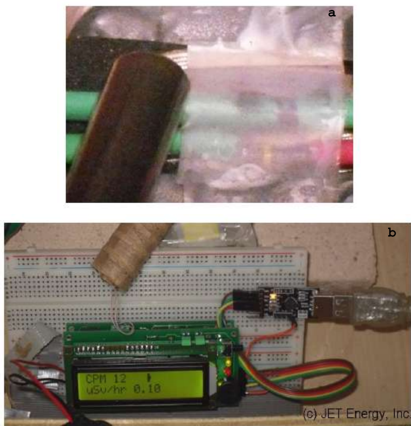
Figure 3. (a) Shown is the central region within the calorimeter. The horizontally directed NANOR-type quantum electronic component, containing active \text{ZrO}_2\text{-PdD} nanostructured material, is located within the upper green cylinder. The Geiger Müller tube is shifted off of the active site (rectangular appearing black area located just above the ohmic resistor (to the right of its yellow-colored band), and off to the right from the center) and shown moved about twice its width to the left from its normal location for the photograph. The Geiger–Müller tube is just outside of the tape and to left for the photograph. In addition, the holders, thermal ballasts, thermal conduction materials, vicinal detectors, and electrical insulation, have been removed to more clearly show this. (b) The modified Arduino delivered 500–700 V to the GM tube while also recording GM output, integrating that to CPM, and a 10 min running average of CPM, and converting to microSv/h. The output was delivering (including tube voltage) to the USB to the second DAQ, and to a charlieplexed digital output over the Arduino (shown with background levels).
