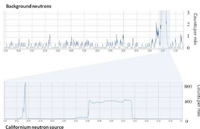
Figure 15. Laboratory background time history ( top ); elevated count rate with a Cf-252 neutron source ( bottom ).
