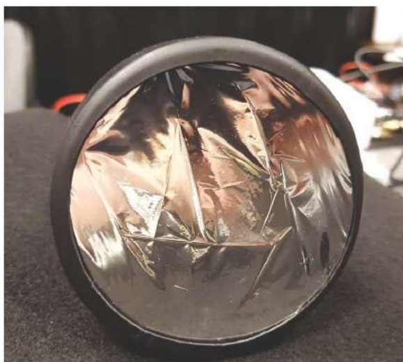
Figure 13. ZnS scintillator/PMT X-ray detector.
