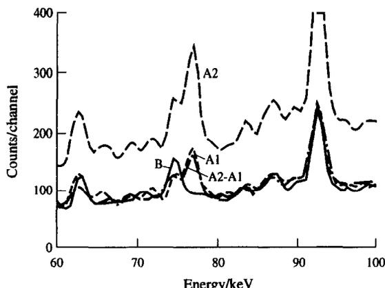
Fig. 3. Gamma ray spectrum before the electrolysis (B) and data are accumulated from 0 to 24 h (A1), and from 0 to 48 h (A2) after electrolysis. (A2-A1) is subtraction from A2 to A1. Gamma ray spectra were obtained by a 4 inch Ge (Li) detector in four shielded containers of 20 cm and 5 mm thick of Pb outer and Cu inner shields. A multi channel analyser of 8000 channels was made to coincide to 0-4000 keV energy range. A gaussian window was fitted for calculation of the spectrum analysis.
